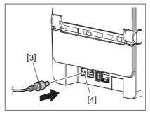
Plug the other end of the power cable into a grounded outlet.
