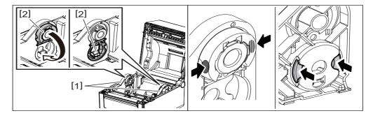
• Printing can be performed with both an outside wound [1] and an inside wound [2] media roll. (Refer to the figure below.) Place the media roll so that its printing surface comes upward.
