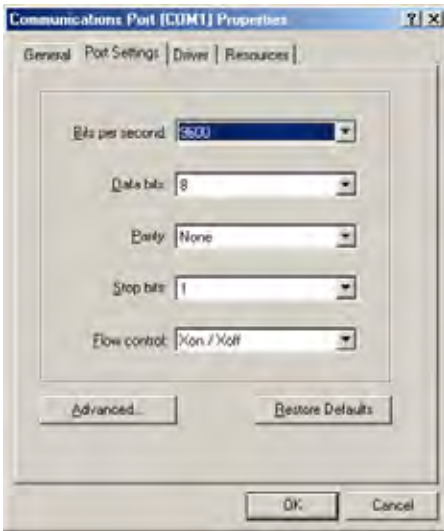
<Reference> Properties screen of Serial (COM) port under Windows98
