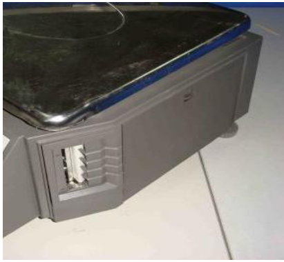
(6) Close the turnable printing assembly.
