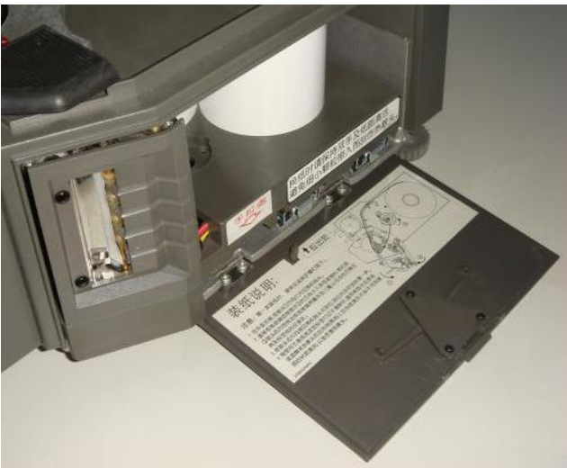
3. Close the rotatable printing assembly
