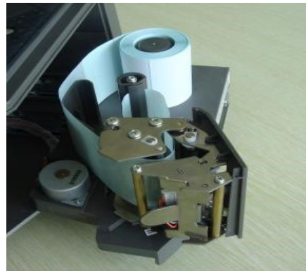
(4) Insert the release paper to the rewriter
